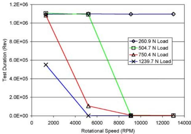
**Fig. 4** Plot of test duration for single round steel washers as a function of load and speed
