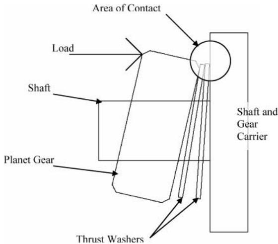
**Fig. 1** Diagram of expected contact loading conditions of thrust washer bearing
