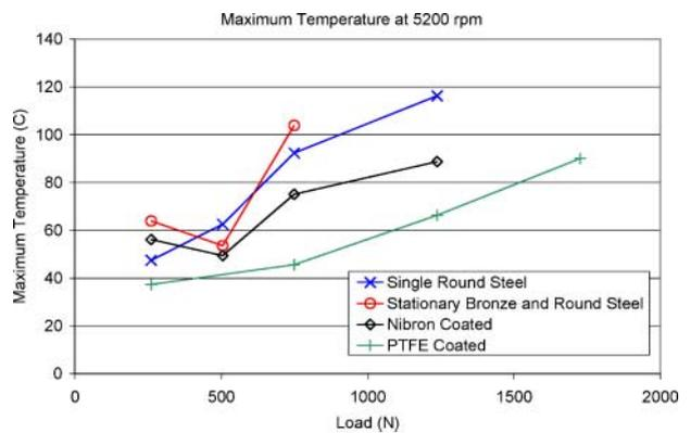
Fig. 19 Maximum bearing temperature plotted as a function of load and washer type
