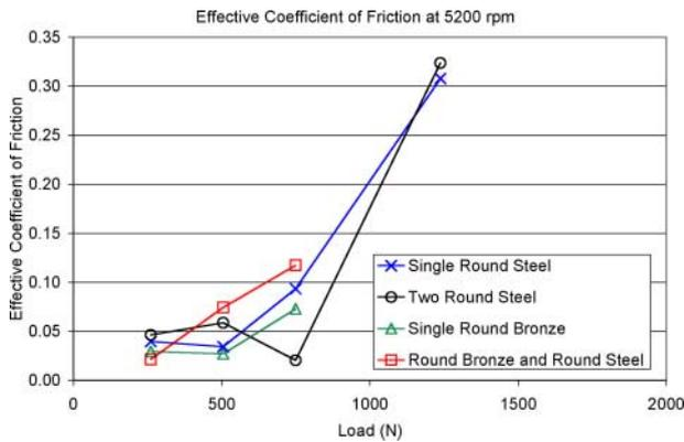
**Fig. 11** Effective COF plotted as a function of load and washer type
