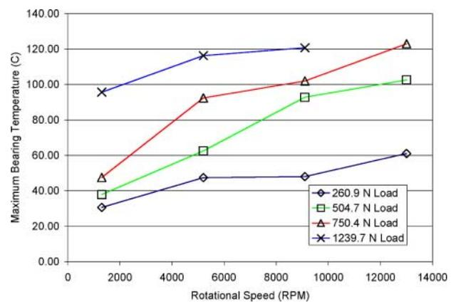
**Fig. 7** Plot of maximum bearing temperature for single round steel washers as a function of load and speed
