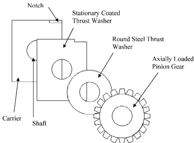
**Fig. 3** Typical coated washer bearing configuration
