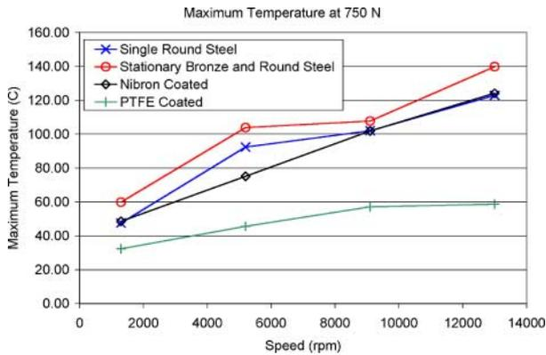
**Fig. 20** Maximum bearing temperature plotted as a function of speed and washer type
