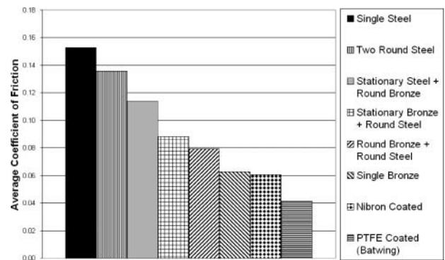
**Fig. 21** The average coefficient of friction for all tests conducted for each washer combination
