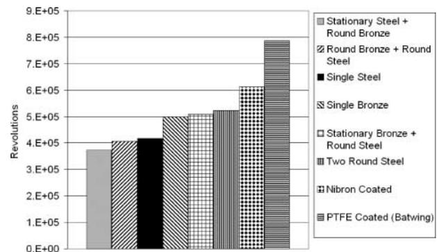
**Fig. 22** The average bearing test duration for each type of tested bearing configuration
