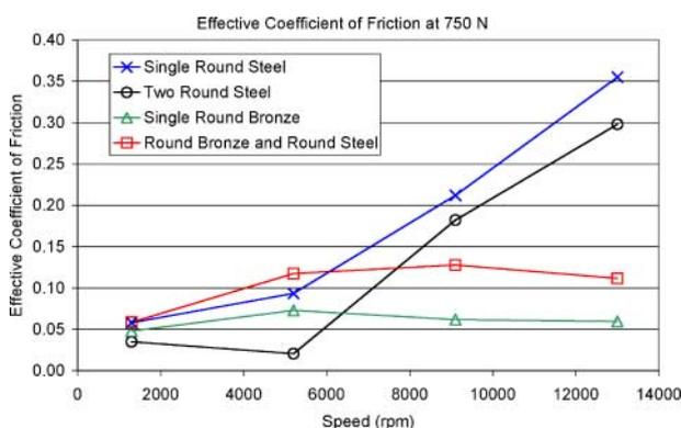
**Fig. 13** Effective coefficient of friction plotted as a function of load and washer type
