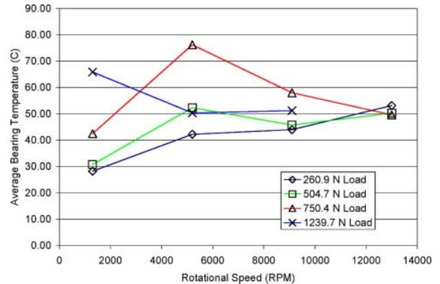
**Fig. 6** Plot of average bearing temperature for single round steel washers as a function of load and speed
