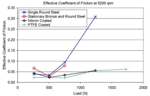
Fig. 17 Effective coefficient of friction plotted as a function of load and washer type
