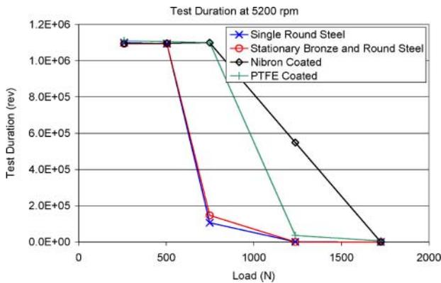
Fig. 15 Test duration plotted as a function of load and washer type
