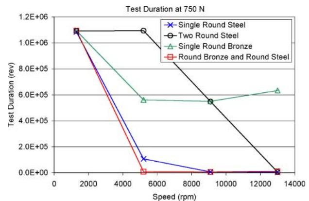
**Fig. 10** Test duration plotted as a function of speed and washer type
