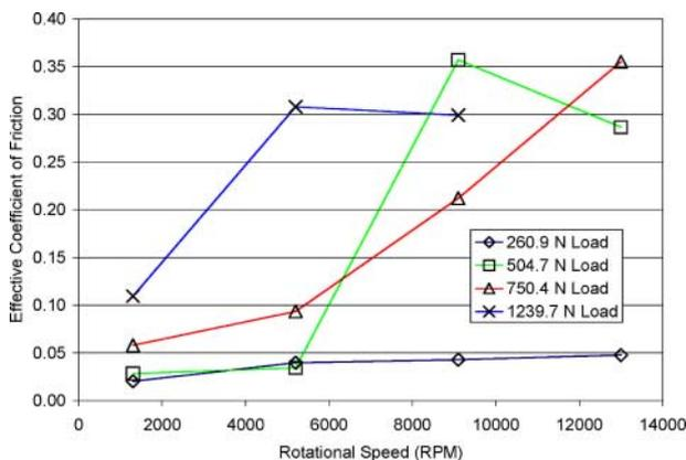
**Fig. 5** Plot of average effective COF for single round steel washers as a function of load and speed
