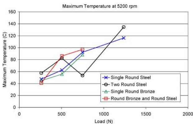
**Fig. 12** Maximum bearing temperature plotted as a function of load and washer type
