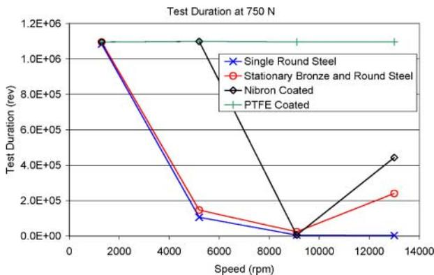
Fig. 16 Test duration plotted as a function of speed and washer type
