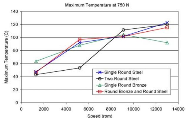
**Fig. 14** Maximum bearing temperature plotted as a function of speed and washer type
