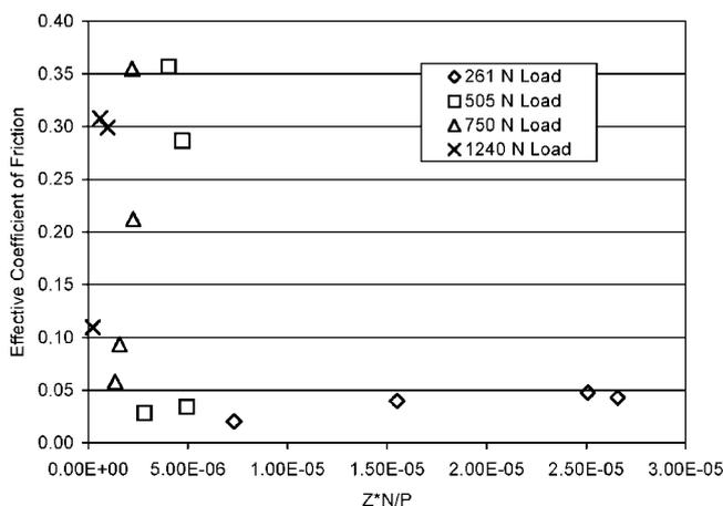
**Fig. 8** Experimentally generated Stribeck plot for a single round steel washer
