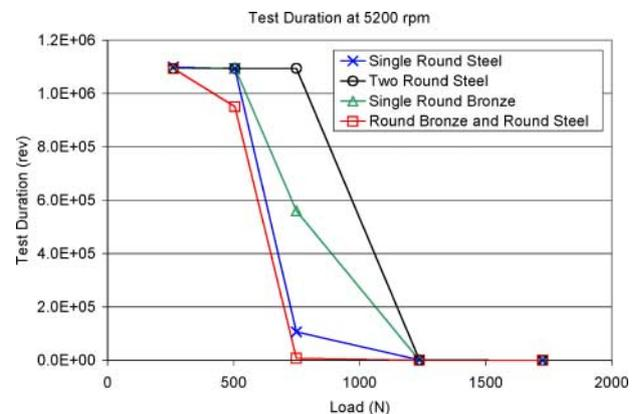
**Fig. 9** Test duration plotted as a function of load and washer type
