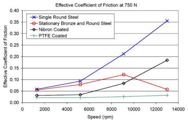
Fig. 18 Effective coefficient of friction plotted as a function of speed and washer type
