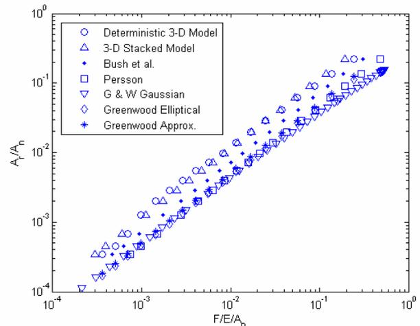
Figure 1: A comparison of real area of contact predictions by several elastic rough surface contact models for the same surface.
