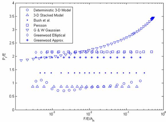
Figure 2: A comparison of real contact pressure predictions by several elastic rough surface contact models for the same surface.
