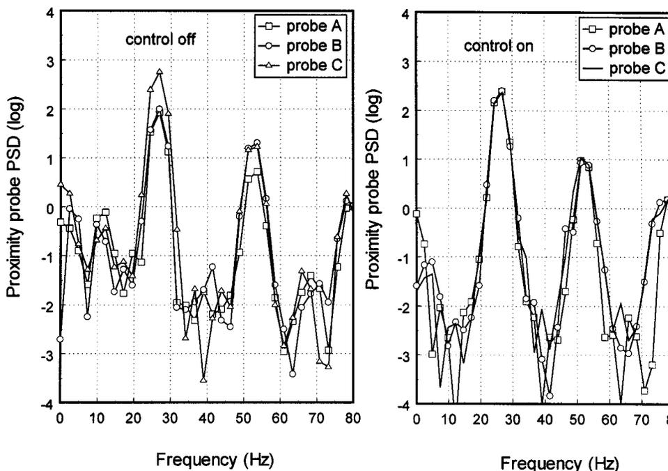
Fig. 7. Proximity probe PSD's when the control is on and off.
