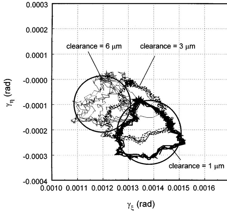
Fig. 3. Rotor angular misalignment orbit (AMO) for different clearances. (Large stator and initial rotor misalignments  $\gamma_s = \gamma_{ri} = 1.5$  mrad.)
