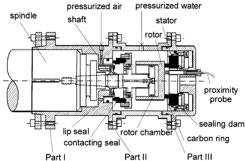
Fig. 2. Schematic of the FMR noncontacting mechanical seal assembly.
