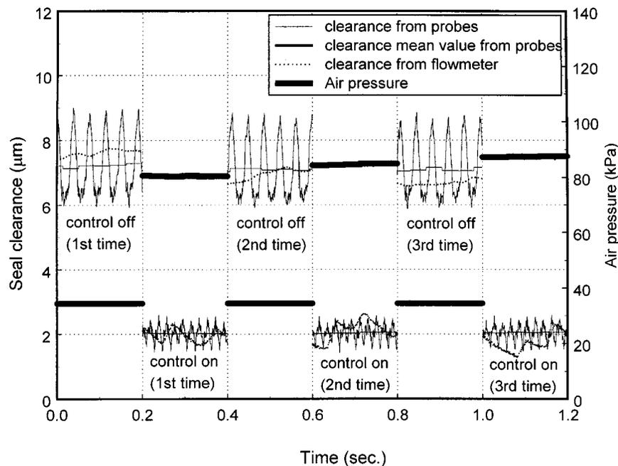
Fig. 10. Seal clearance and air pressure when the control is on and off.
