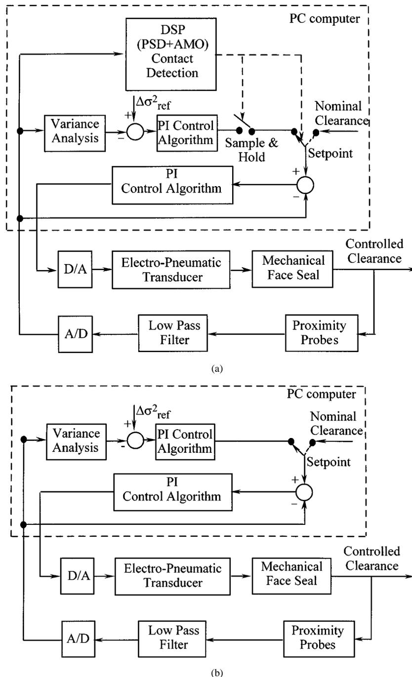
Fig. 4. Block diagram of the seal clearance control system. (a) Supervisory control using DSP and AMO analysis to detect contact. (b) Continuous supervisory control using variance analysis to detect contact.
