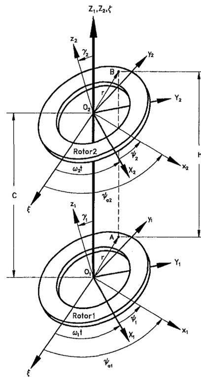
Fig. 2 FMRR seal kinematic model and coordinate systems
