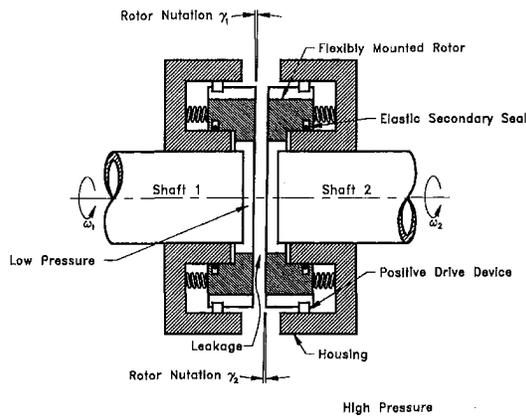
Fig. 1 Schematic of an FMRR mechanical seal
