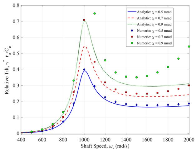
**Fig. 3 Comparing the numeric solution of the full nonlinear equations of motion to the analytic solution of the linearized equations of motion ( $\delta = 2$ )**
