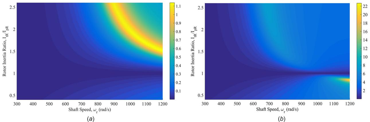
**Fig. 7 Relative tilt versus shaft speed  $\omega_r$  and rotor inertia ratio  $\delta = I_{tr}/I_{pr}$  ( $\chi = 0.5$  mrad): (a) case when the rotor inertia is much larger than the FMS ( $I_{tr}/I_{ts} = 50$ ) and (b) case when the rotor inertia is comparable to the FMS ( $I_{tr}/I_{ts} = 2$ )**
