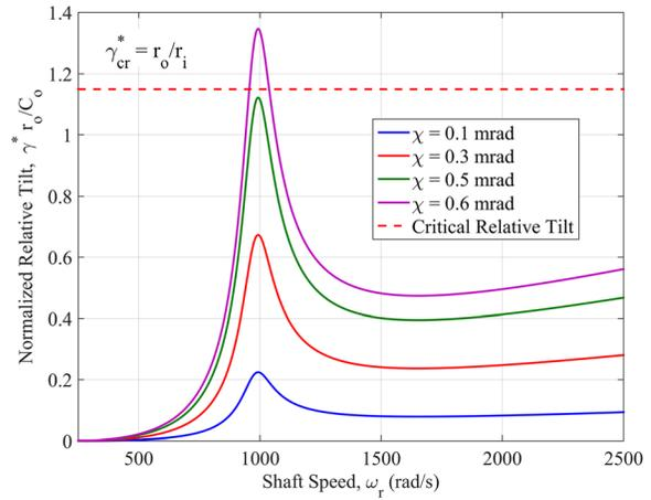
**Fig. 6 Relative tilt versus shaft speed for several values of angular misalignment, highlighting the appearance of face contact when coupled rotordynamics are included ( $\delta = 2$ ,  $I_{tr}/I_{ts} = 50$ )**
