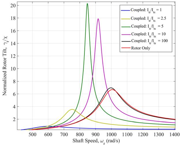
**Fig. 4 Investigating the influence of FMS dynamics on rotor response for an angular misalignment of  $\chi = 0.5$  mrad,  $\delta = 2$**
