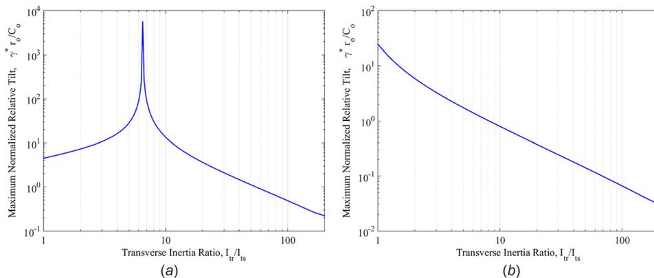
**Fig. 5 Relative tilt versus rotor–stator inertia ratio for thin and thick rotors: (a) thick rotor ( $\delta = 2$ ) and (b) thin rotor ( $\delta = 0.5$ )**
