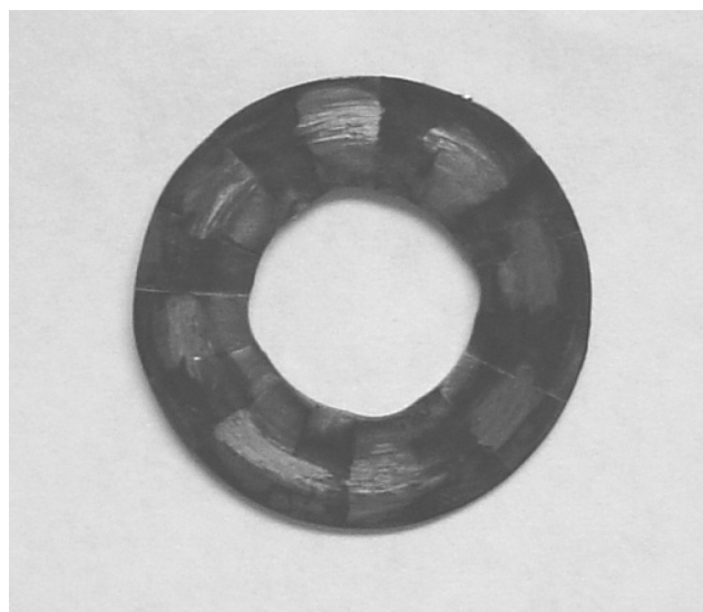
Fig. 6—Picture of worn grooved washer after run for procedure 1.
