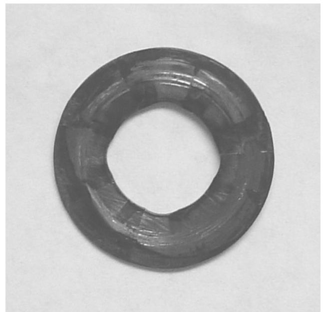
Fig. 9—Picture of worn grooved washer after run for procedure 2.
